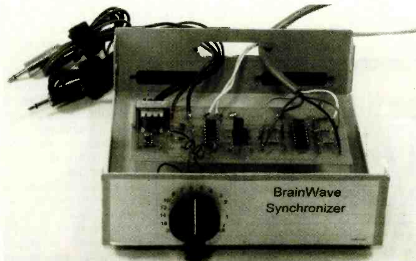
Fig. 5. The completed Visual Brainwave Synchronizer fits nicely into a computer port switchbox. The switchbox's knob can be recycled for turning R12.
